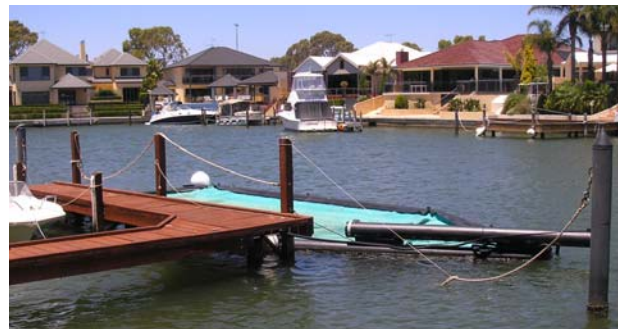
Seapens have significant advantages and avoid the need to anti-foul permanently moored vessels.
